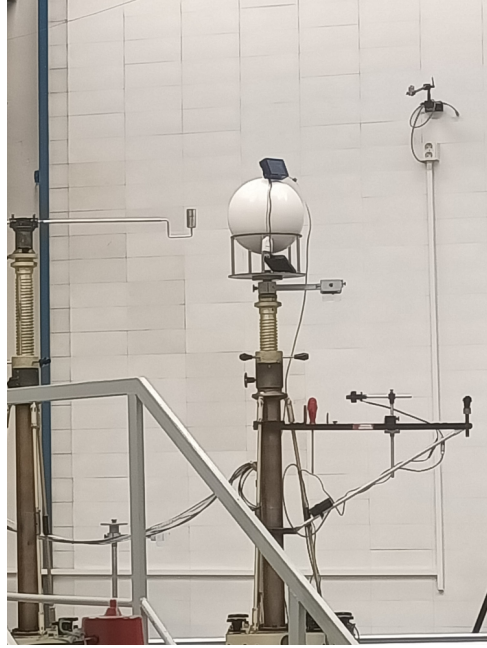
Figure 3.20: Positioning of rem counter in CMI calibration room with the Am-Be source.
