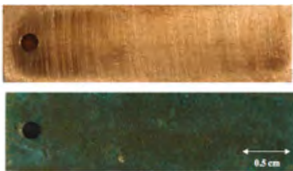
Figure 2. Bronze ingot before and after the corrosion test.
