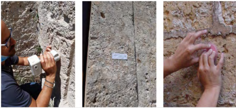
Figure 15. Non-invasive and cost-effective diagnostics to evaluate products behaviour. Colorimetric Test on the left; Scotch Tape Test in the middle; Water Absorption on the right.
