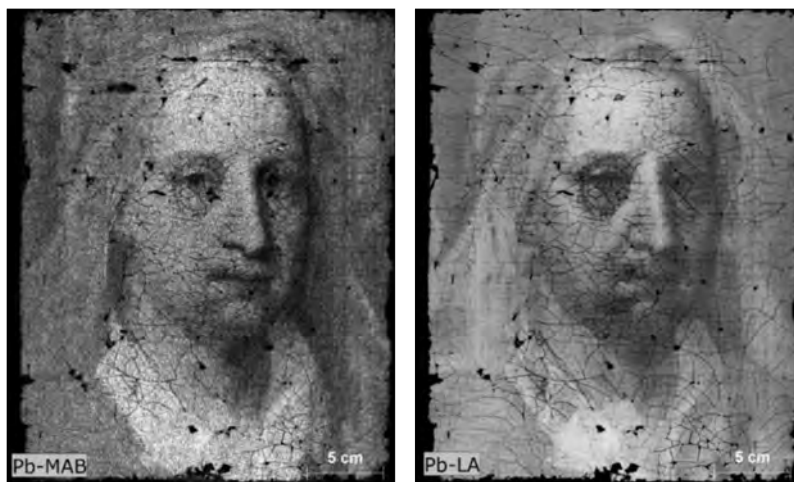
Figure 1. These element distribution images shown the distribution of lead in a painting. The first image shows the Pb-M lines at 2.4 keV and the second the Pb-La line at 10.54 keV. The difference in energies allows “display” of the element distribution at different depths. The L lines show the painting down to the grounding, including the damaged areas on the left side, and the M-lines show the topmost thin layers of Pb pigments present at the painting’s surface (Tagle Berdan et al., 2019 and references therein).
