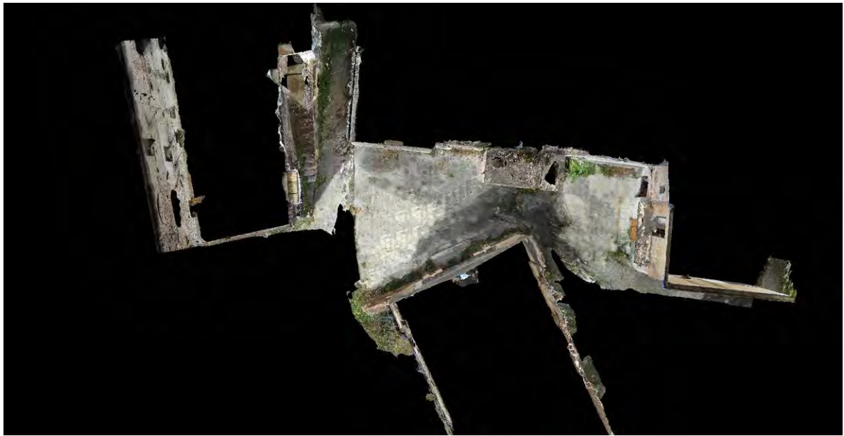
Fig. 7: Photogrammetric model of Alianello.
