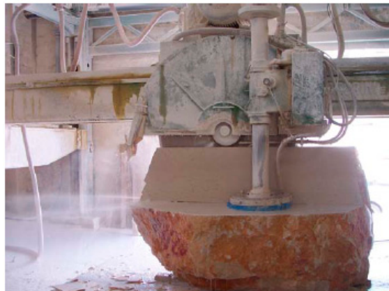
Figure 2. The tool with a water-cooled diamond blade during the processing of Apricena limestone block.
