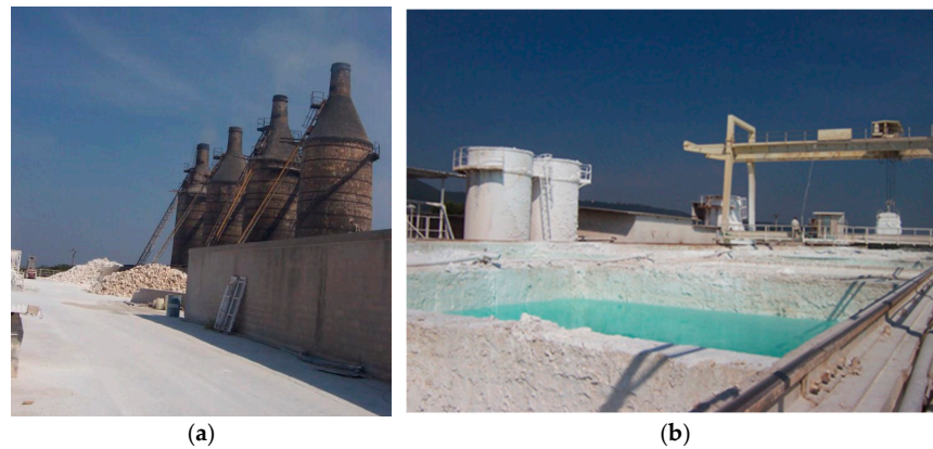
Figure 1. (a) Vertical kilns for the production of quicklime; (b) Tanks of quicklime slaking and long-term aging of lime putty.
