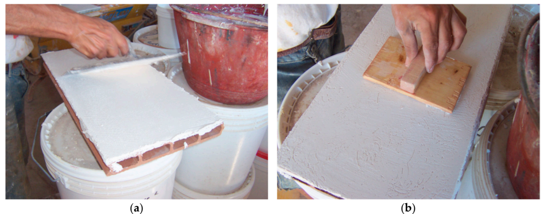
Figure 12. Applicability test of white fine mortar. First layer of finishing plaster applied with steel trowel (a), surface treatment with a small wooden trowel (b).
