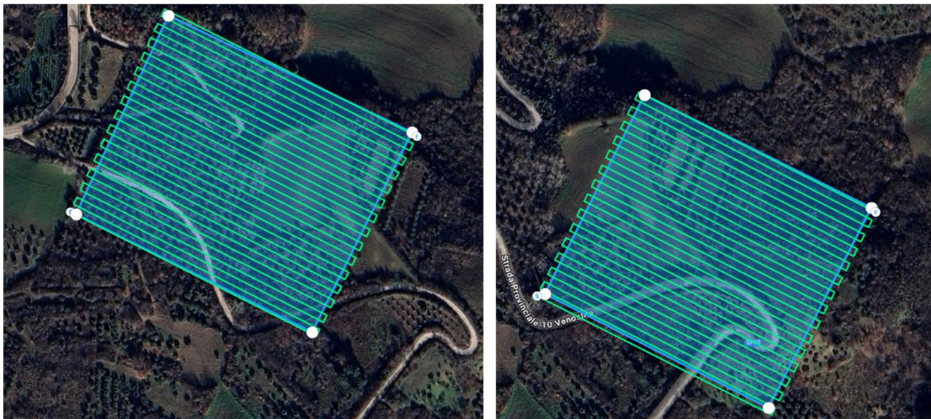
Fig. 2 The two flight plans considered during the acquisition of visible and thermal images. Cyan rectangles indicate the areas acquired by the UAV surveys and the green lines represent UAV flight paths
