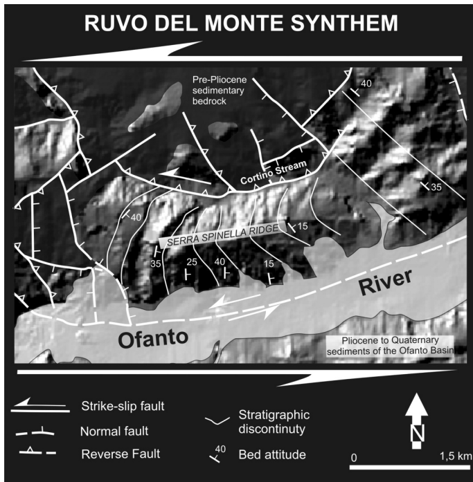
Fig. 13 - Geometrical sketch of the Serra Spinella ridge. The progressive unconformities of the growth structure and the dip directions of the single sedimentary bodies are the result of an E-W oriented left-lateral strike-slip motion, as also shown by the complex fault association at the northern basin boundary.
