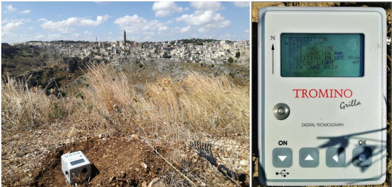
Fig. 2.22 TROMINO digital tomograph used in recording.
