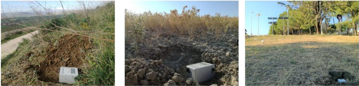
Fig. 2.15 Different criterion for single station ambient noise measurement: (left) removing vegetation and firm embedding of the instrument's feet in the ground before measurement protecting it from wind; (centre) levelling of the sensor on the surface of the measuring point, especially in steep topographical conditions; (right) moving the measurement point away by a distance at least equal to the height of the nearest structure (trees and light poles in photo) to trying to follow the requirement of free-field soil condition
