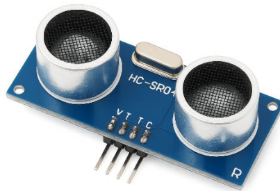
Figure 4.3. HC-SR04 ultrasonic distance sensor module (AI-Generated Image).
