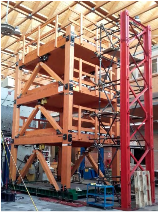
Figure 3: Experimental post-tensioned timber frame model tested at the structural laboratory of University of Basilicata.
