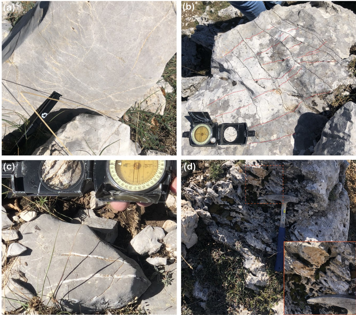
Figure A.10 (a) Sheared veins collected at the vicinity of the N-S inferred fault bounding block A and block B. (b) Mutual crosscutting relationships between veins oriented N110 - N120 and those oriented N30 - N40. These veins are abundant throughout the study outcrops. (c) 4mm-thick veins as observed within the N-S inferred fault zone. (d) Brecciated rocks collected along the N-S inferred fault zone.
