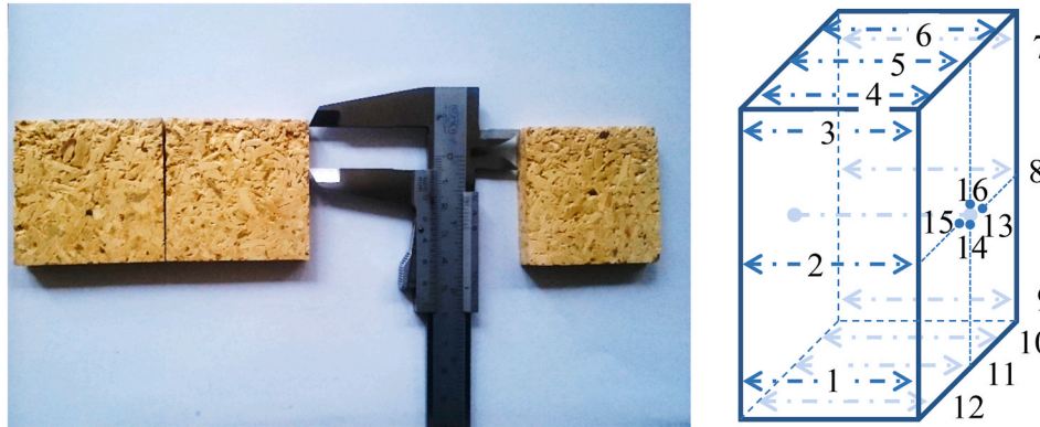
Fig. 2. The sample set on the left and the schematic diagram of the sample part showing all the points used for measuring the thickness dimensions is shown on the right.
