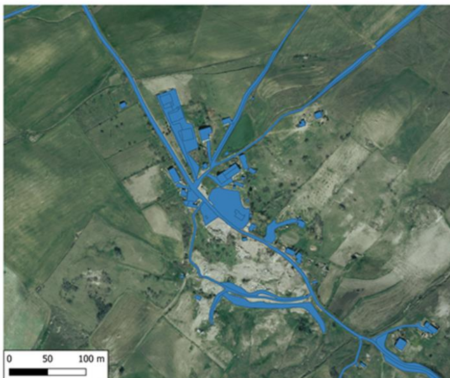
Figure 21. Detail of the urban agglomeration (Via Bosco Piccolo - Municipality of Potenza) destroyed by the 2013 landslide. In blue the information layers of the GTDB of the Basilicata region regarding the waterproof areas.
