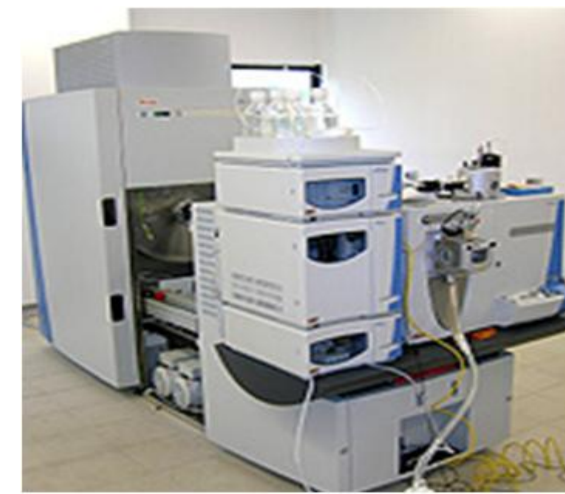
HPLC-DAD and LC system coupled to a hybrid LTQ-FTICR (7-T) mass spectrometer (MS)
