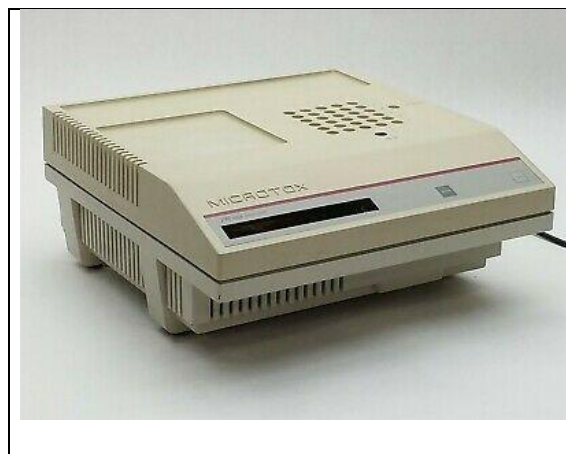
Figure 30 – M500 luminometer used in the execution of the tests (Photo AZUL Environmental. Strategic Diagnostics Inc. Newark, USA)
