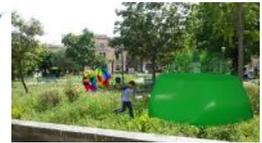
The bubble will be illuminated by a lamp powered by a flexible solar panel. It will consist of two materials: metallic polyester externally, to protect from weather conditions; pvc internally, to protect against UV rays and humidity; between the two materials, a hollow space of compressed air fed by an electric motor.
