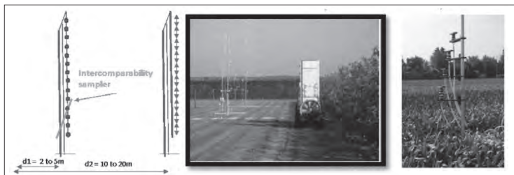
Standard protocol for measurement of pesticide emission to the air
