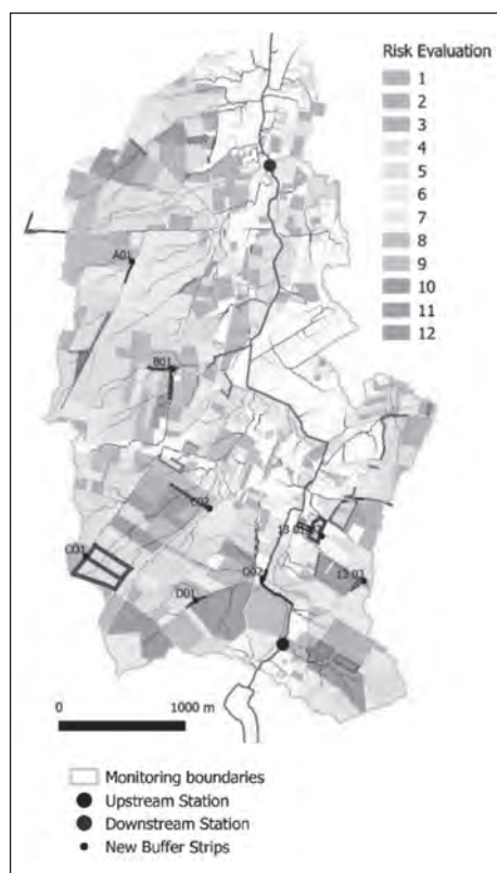
Additional buffer strips implemented after risk evaluation of the catchment
