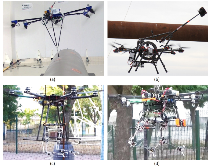
Fig. 1. AEROARMS platforms: (a) Multi-directional thrust hexarotor with a rigidly attached end-effector; (b) Multi-directional thrust octorotor with an inspection arm; (c) Aerial dual-arms manipulator with stiff joints; (d) Aerial dual-arms manipulator with compliant joints
