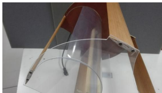
Figure 8. A detail of the investigated hybrid turbine Darrieus-Savonius, with the Darrieus blades at 2/3 of the maximum extension.
