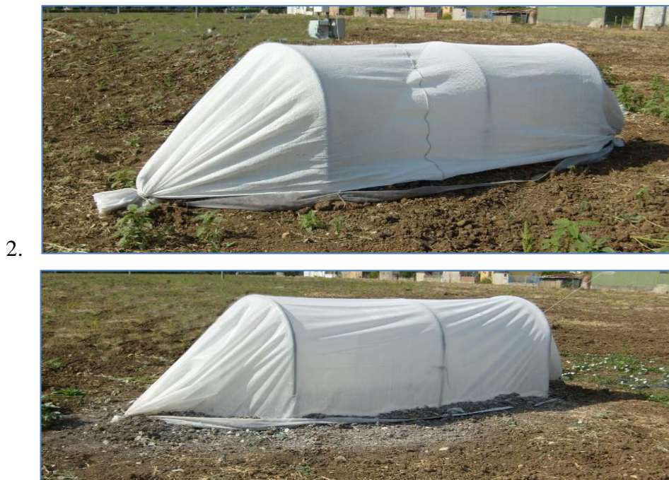
Figure 2.1: Trial small-scale tunnel covered with a 60% shading net adhering to the EVA film (left) and with the same EVA film whitened with Calcium Oxide (right)
